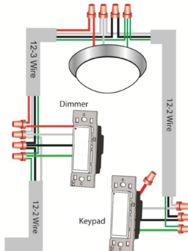
Three-Way with Load at Beginning of Circuit
