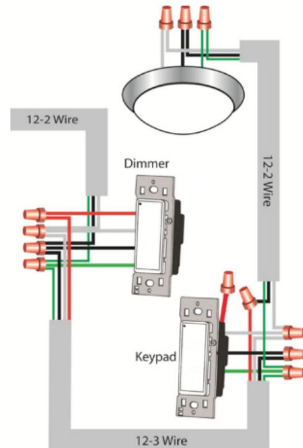
Three-Way with Load in Middle of Circuit
